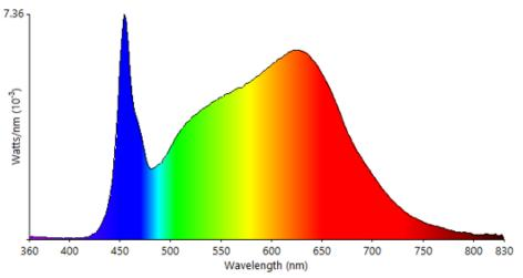
Testing was performed in accordance with LM-79-08.
